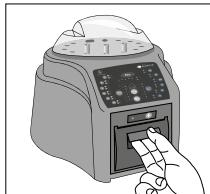
1. To replace the paper roll, pull the handle of the printer's door.
