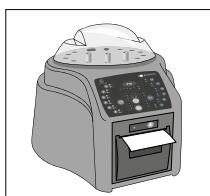
4. Close the printer cover by pressing on the sides of the lid.
