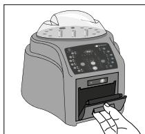
2. Open the printer's cover and remove the spent roll.
